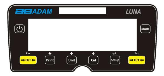
The keypad has the following keys to operate the balance.
