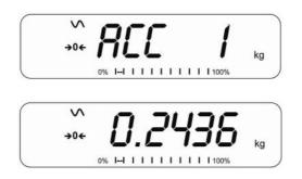
• When the scale is at zero place a second weight. Press [Print] to accumulate the weight. Remove the weight and press [Print]. The display will show "ACC 2" for 2 seconds and then show the new total.
