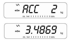
• Continue until all weights have been added. This can continue for up to 99 entries until the capacity of display is exceeded.
